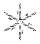
azimuth, oriented from magnetic north. Used as the basis for navigation in the national airspace system. The VOR periodically identifies itself by Morse Code and may have an additional voice identification feature.
